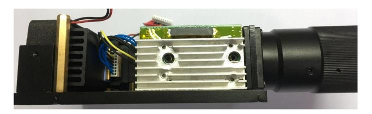
• 4. Remove DMD Heat-sinking , leaf spring ; DMD board
